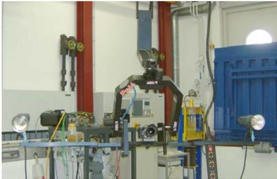
Image 3: Remote controlled 3D- head *Pele XL* from *MovieTech*, Munich, Germany with the new constructed bar for the flash heads, during lab tests.
