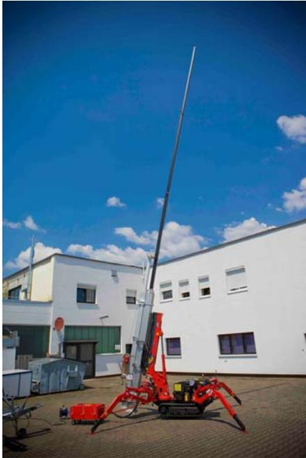
Image 2: The *Unic* Minicrane is the base for the RRS system. It is adapted with a newly constructed 25m boom. On the end of the boom a remote controlled 3D head can hold either the digital camera with the two flash heads or optional various recording systems. The image shows the system while in construction; first tests were restricted to 15m.
