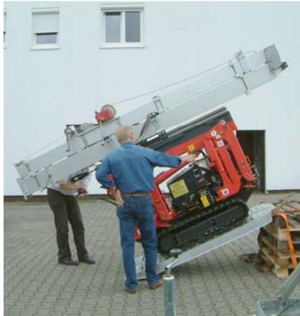
*Image1: RRS System during construction. The tests for climbing inclines in compact Transport modus shows, that the System is able to overcome up to 21 degree on ramps.*
